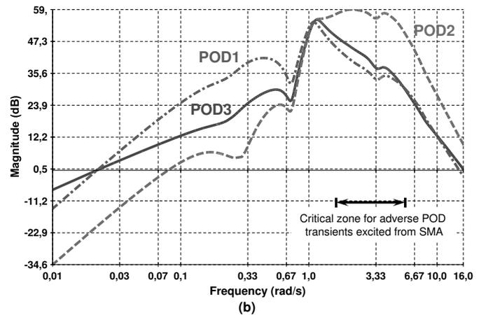
Fig. 13. Bode magnitude plots of the closed-loop disturbance channel for Scenario I:  $POD_1$ , dash-dot;  $POD_2$ , dashed; and  $POD_3$ , solid; (a)  $B_{SC}(j\omega)/P_{mec}^{TUC}(j\omega)$ ; (b)  $B_{SC}(j\omega)/P_{mec}^{SMA}(j\omega)$ .
