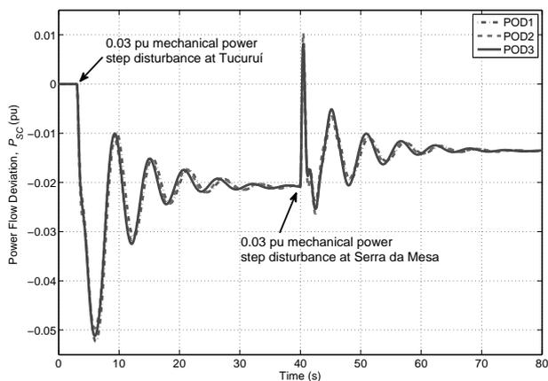
Fig. 15. Line power transients ( $P_{SC}$ ) following step disturbances  $P_{mec}^{TUC}$  (at 3s) and  $P_{mec}^{SMA}$  (at 40s) for Scenario I, refer to Fig. 2.
