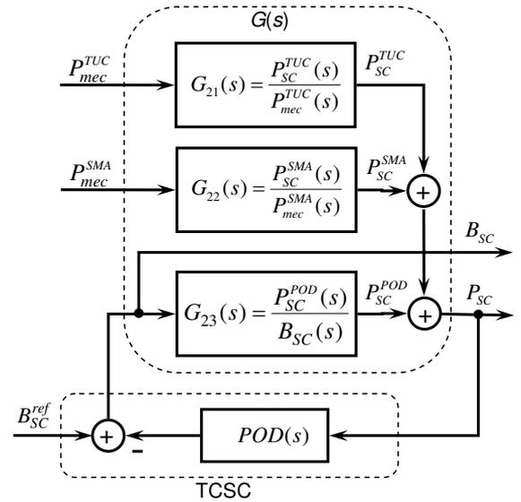
Fig. 3. BIPS model used for robust POD controller analysis and design.
