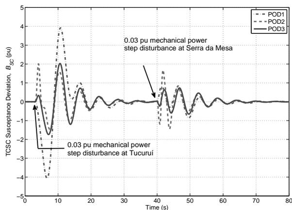
Fig. 16. Transients in  $B_{SC}$ , the TCSC effective susceptance, following step disturbances  $P_{mec}^{TUC}$  (at 3s) and  $P_{mec}^{SMA}$  (at 40s) for Scenario I, refer to Fig. 2.
