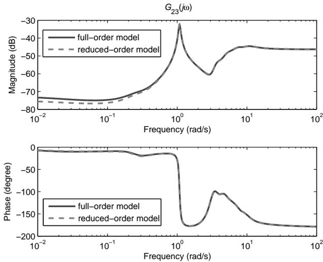
Fig. 6. Bode plots for  $G_{23}(s)$  considering the full BIPS model (1,664 states) and the reduced 200-state model (Scenario I).
