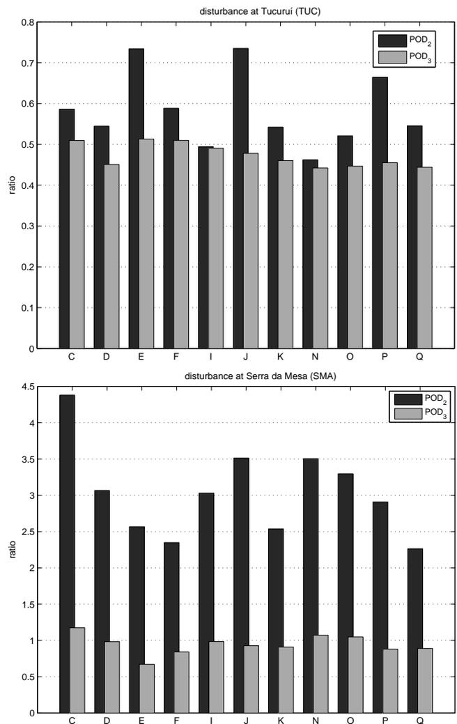
Fig. 17. Ratios between  $B_{SC}$  transient peaks ( $POD_{2,3}/POD_1$ ) following an applied step in the disturbance channels.
