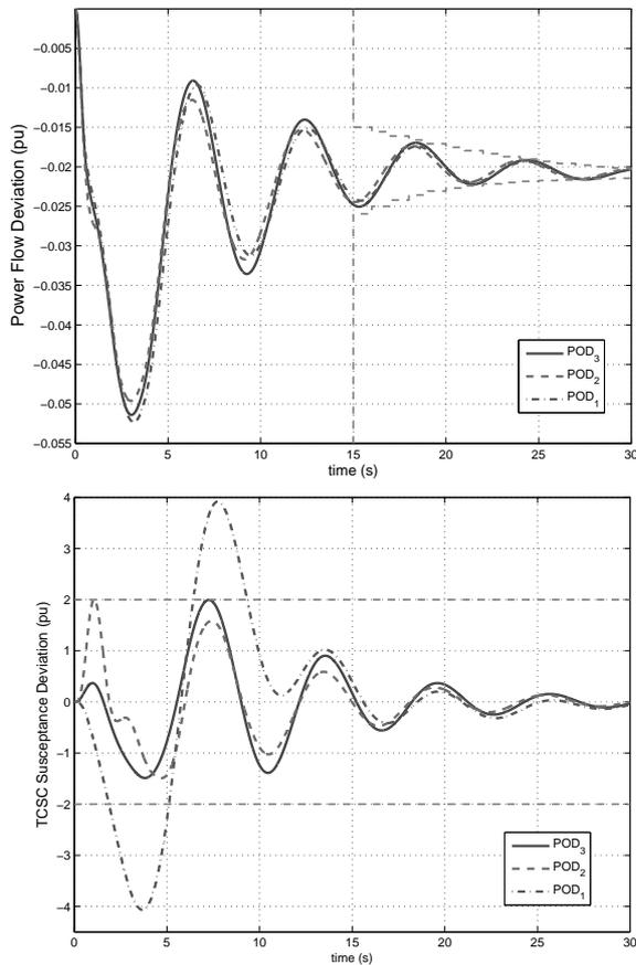
Fig. 10. Linear simulations for disturbance at Tucuruí (Scenario I).
