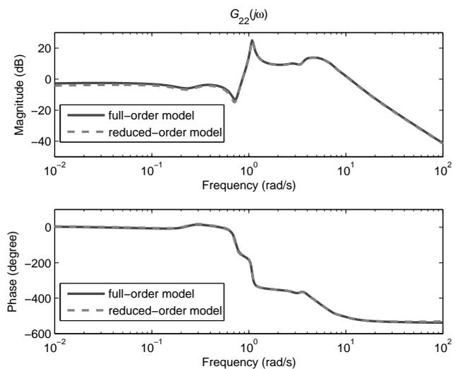
Fig. 5. Bode plots for  $G_{22}(s)$  considering the full BIPS model (1,664 states) and the reduced 200-state model (Scenario I).
