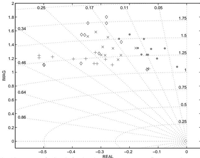
Fig. 12. Locus of NS pole for the eleven nonzero power flow scenarios: open-loop (dot-mark), closed-loop for  $POD_1$  (x-mark), closed-loop for  $POD_2$  (plus-mark) and closed-loop for  $POD_3$  (diamond-mark).
