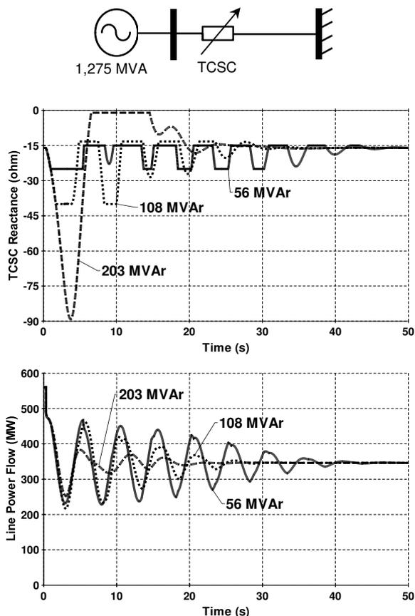
Fig. 1. Impact of TCSC limits on the power flow oscillation damping of a single machine-infinite bus example.
