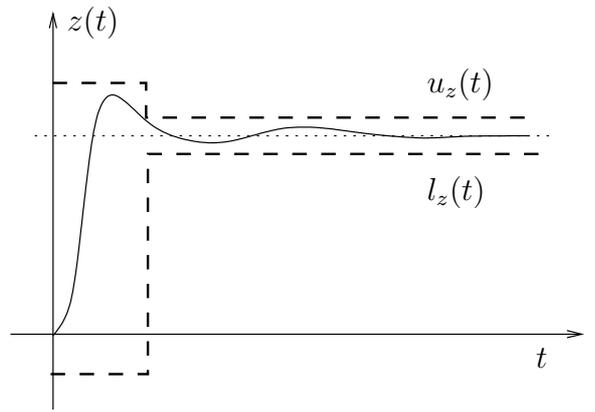
Fig. 7. Shape-constraints on the step response
