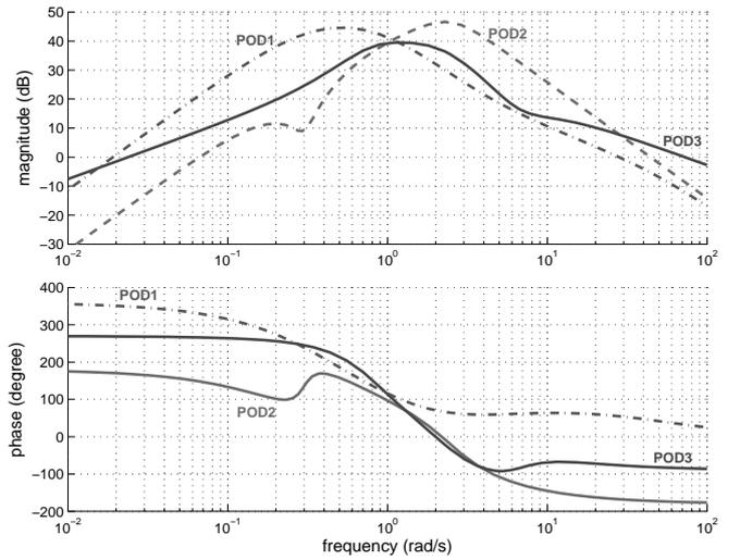
Fig. 9. Bode plots for the phase-lag ( $POD_1$ , dash-dot), phase-lead ( $POD_2$ , dashed) and nonsmooth ( $POD_3$ , solid) PODs.
