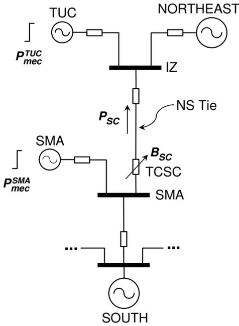
Fig. 2. Schematic diagram of Brazilian Interconnected Power System (BIPS) in year 1999. Acronyms SMA, TUC, IZ denote Serra da Mesa, Tucuruí and Imperatriz power plants or substations.
